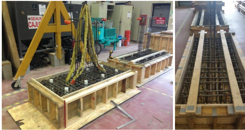
Figure 24 - Reinforcement cage in wooden formwork
