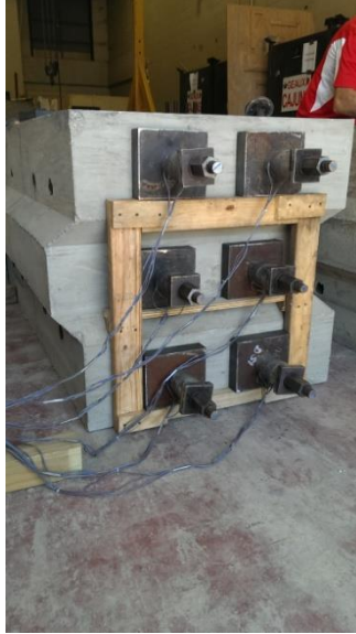
Figure 40 - DYWIDAG bar locations
